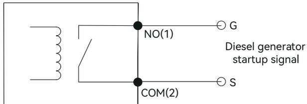
Figure 5-26 Generator Control connection diagram
