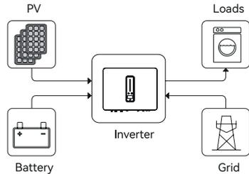
**Peak load Shifting (Load Shifting)**
